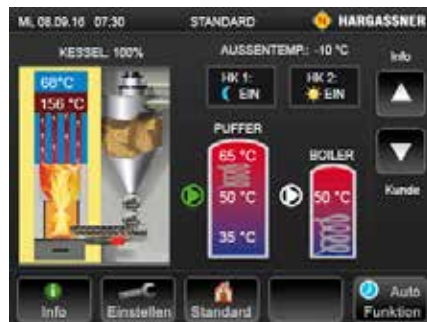
Boiler in Full-Load: Display shows a working boiler. HWT and Accumulator are being loaded already. Heating Circuits ensure required temperature in each living-area.
