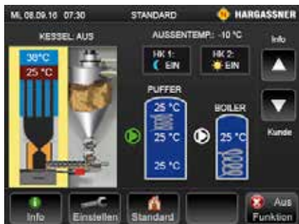
KeBoiler before starting: Display of Lambda Touchtronic shows a not-heated boiler. HWT and Accumulator are cold - not loaded
